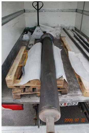
Radiant Tube coated with sintered Emisshield® Product
